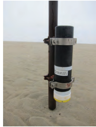
Fig. 1. One of Engelstad's wave gauges positioned on beach at Schiermonnikoog, December 2016. This gauge is "a submersible self-logging, self-powered pressure sensor. It combines a temperature compensated, highly stable, pressure sensor, a Compact Flash Card Data Logger, a rugged waterproof package and 12 C size Alkaline Batteries." Description taken from the Ocean Sensor Systems website ( http://www.oceansensorsystems.com/products.htm ). Photograph by author.
